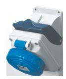
Compact industrial socket-outlets complying with the IEC 60309 Standard (EN 60309-1 EN 60309-4), with more simple and intuitive longitudinal operation of the mechanical interlock. The control switch allows the plug to be connected and disconnected only in the open position, and the switch to close only with the plug interlock switch is combined with a complete range of accessories for individual or group surface-mounting, and for flushmounting (also possible on 3 gang rectangular boxes).
